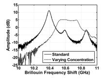
Fig. 2. Area normalized Brillouin gain spectra for standard and varying concentration phosphosilicate fibers.
