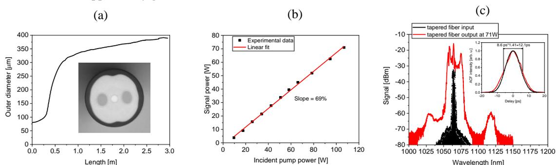
**Fig. 1** (a): dependence of outer diameter on the tapered fiber length (inset: fiber cross section photo); (b): output signal power on incident pump power dependence; (c): signal spectra at the tapered fiber input (black) and tapered fiber output at 71 W average power (red) (inset: autocorrelation functions before and after tapered fiber at 71 W average power).
