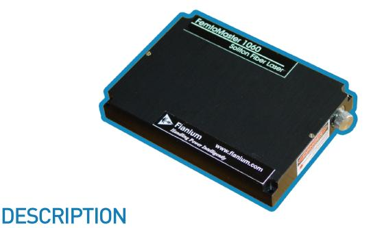
FemtoMaster is a passively mode-locked soliton fibre laser with a semiconductor saturable absorber as one of the cavity mirrors. The active medium is a core-pumped Yb-doped fibre. The laser oscillators generate transform-limited 3-6 ps pulses. Systems generating more than 10 mW of output power as also equipped with a fiber amplifier.
